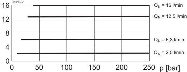
$\Delta p = f(Q)$  Pressure loss/flow characteristics
