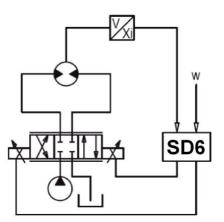
• Controller mode –5 "Pressure control closed loop (2-sol)"
