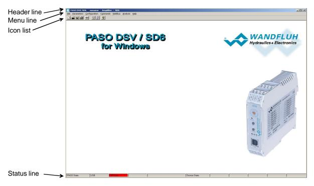
During the start-up, the parameterisation software PASO DSV/SD6 checks, whether a Wandfluh-Electronics device is connected. If no communication can be established, an error message appears (refer to section "Communication interruption" as) and the "Off Line"-mode will become active. All menu points and keys, which involve an action in connection with the communication, are then blocked. All other functions of the parameterisation software PASO DSV/SD6 can be utilised without any limitation.
