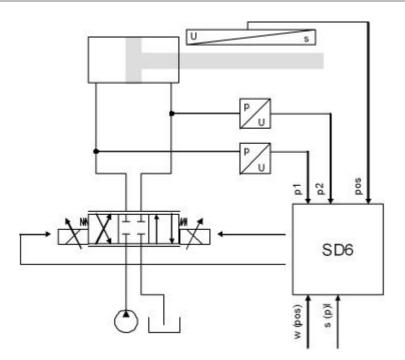
This setting is available only with a SD6-electronics with software version higher than 1.1.3.0 and PASO with software version higher than 1.5.1.2!
