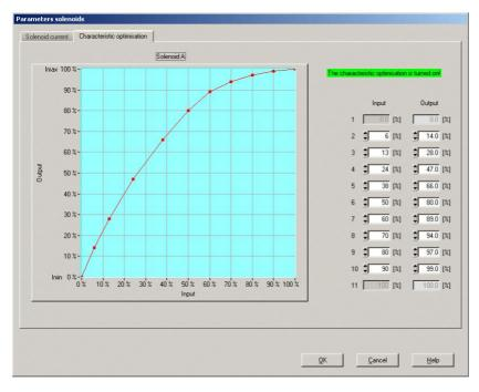
The solenoid current values are in the range Imin (0%) up to Imax (100%). Imin and Imax are adjusted in the
