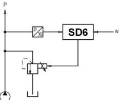
Example Application: Flow Control: with one proportional throttle valve, the flow Q is held constant to the flow command value w.
