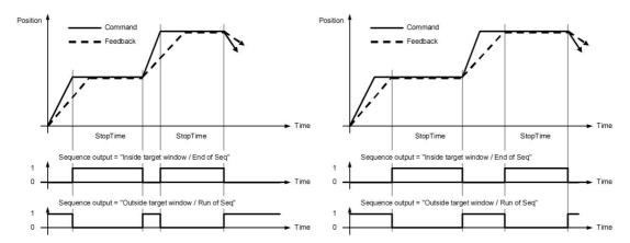
From the travel command data, the theoretical course of the sequence is calculated. The calculated course of the sequence is jointly determined by the limit parameters (position and speed at the beginning and end of the sequence) and it can significantly differ from the travel command data entered. Command positions and possible stop times, however, are complied with in all cases.
