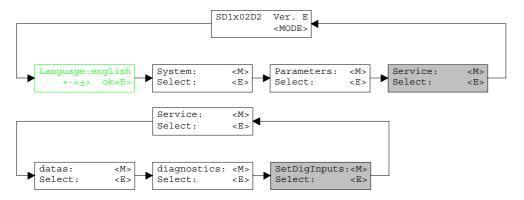
With this command, the digital inputs of the connected Amplifier can be set to active, not active or released.
