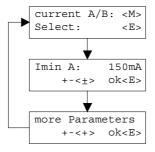
With the keys "+" and "-", the desired value can be adjusted. With the key "ENTER", the next parameter value will be displayed. All existing parameters are listed in the section "Settings" page 17 with the column "Field".
