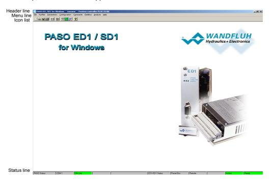
During the start-up, the parameterisation software PASO checks, whether a digital controller card is connected. If no communication can be established (communication interference or no axis controller connected), an error message appears. All menu points and keys, which involve an action in connection with the communication, are then blocked. All other functions of the parameterisation software PASO can be utilised without any limitation.
