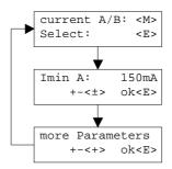
With the keys "+" and "-", the desired value can be adjusted. With the key "ENTER", the next parameter value will be displayed. All existing parameters are listed in the section "Settings" page 24 with the column "Field".
