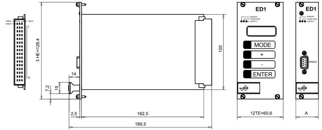
A: 6TE = 30.1mm for the 10-Bit card 10TE = 60.6mm for the 12-Bit card
