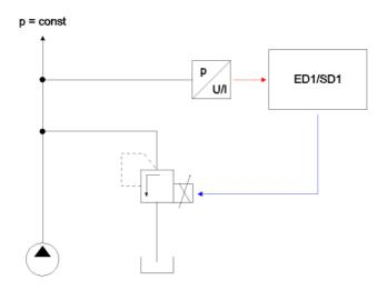
This system is actual only a electronically preset value re-lead. The problem is, that the pressure already is mechanical controlled inside the valve. Because this mechanical control is very slow, the electronically control must be made slow artificially (cascade control: the exterior loop must be slower than the interior loop). With such a system, good static requests can be performed. However, dynamic requests can be bad performed.
