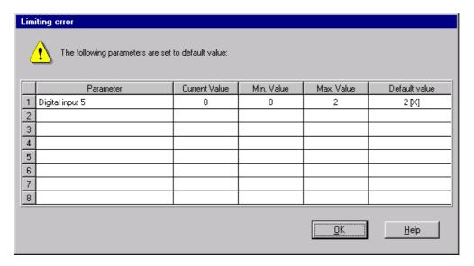
Parameter: Name of the parameter with the limiting value error
