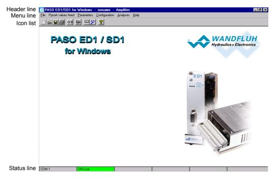
During the start-up, the parameterisation software PASO checks, whether a digital controller card is connected. If no communication can be established (communication interference or no axis controller connected), an error message appears. All menu points and keys, which involve an action in connection with the communication, are then blocked. All other functions of the parameterisation software PASO can be utilised without any limitation.
