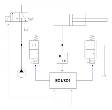
This system correspond to the pressure reducing with throttel valves function (refer to section "Pressure reducing control with throttle valves (2-solenoid application)" page 10.
