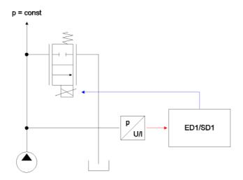
With this system, high dynamic and static requests can be performed. Any proportional valves with one active control edge can be used. Recommended valves: D.PPM18, D.PPM22, D.PPM33
