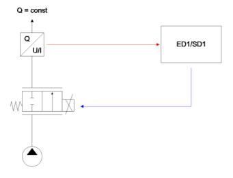
With this system, high dynamic and static requests can be performed. Any proportional valves with one active control edge can be used. Recommended valves: D.PPM18, D.PPM22, D.PPM33
