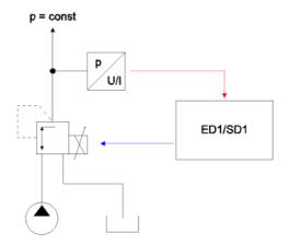
This system is actual only a electronically preset value re-lead. The problem is, that the pressure already is mechanical controlled inside the valve. Because this mechanical control is very slow, the electronically control must be made slow artificially (cascade control: the exterior loop must be slower than the interior loop). With such a system, good static requests can be performed. However, dynamic requests can be bad performed.
