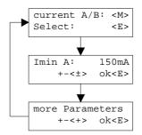
With the keys "+" and "-", the desired value can be adjusted. With the key "ENTER", the next parameter value will be displayed. All existing parameters are listed in the section "Settings" page 16 with the column "Field".
